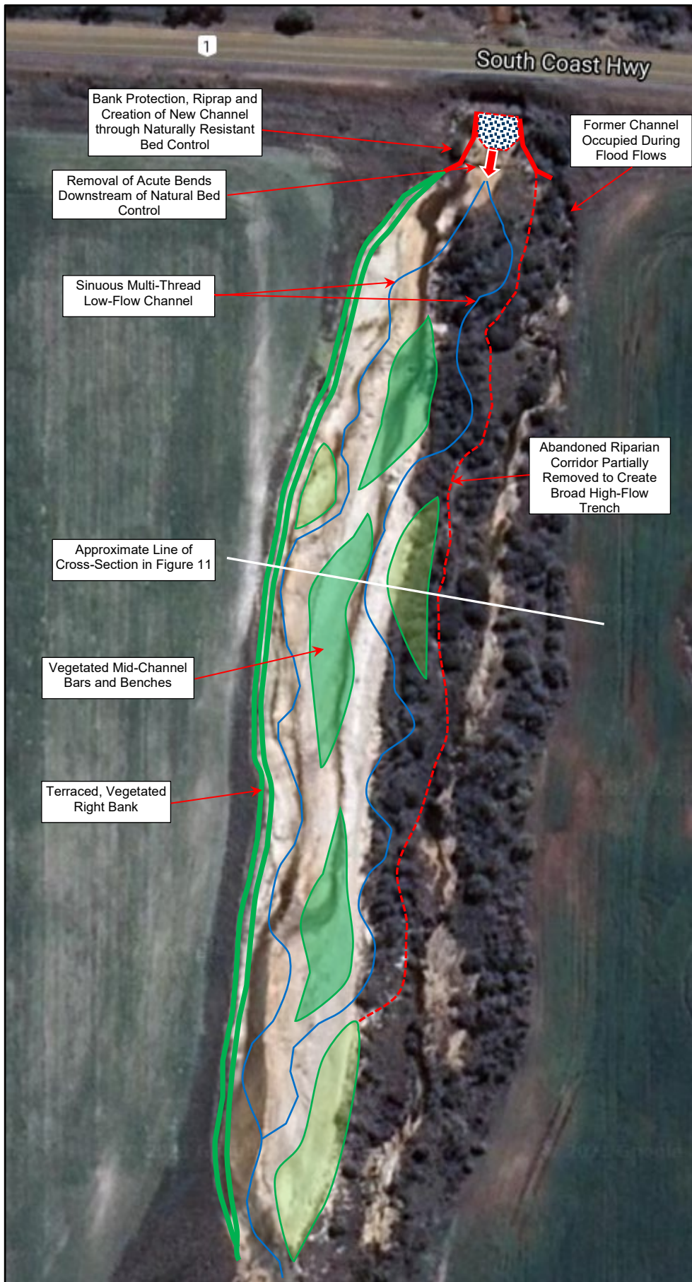
Figure 10 Conceptual remediation design planform of Coobidge Creek
